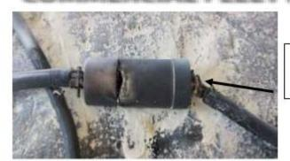
The electrical plugs that shorted out causing an arc flash. (Notice the poor wiring at the extension cord's receptacle.)
